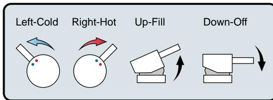
**CAUTION:** There is no automatic shut off with the water fill valve. You **MUST** turn the valve OFF after the tub is filled to prevent overflow and/or flooding. Do not walk away from the tub while it is filling with water.
