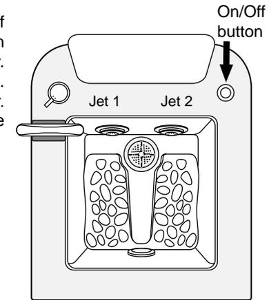
**WARNING:** Running the jets without filling the tub with water can damage or destroy the jets. Ensure that a minimum of one (1) inch of water is above the jets prior to use.
