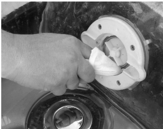
Clean back of screen Jet with same soft brush or cloth. Rinse with cold water
