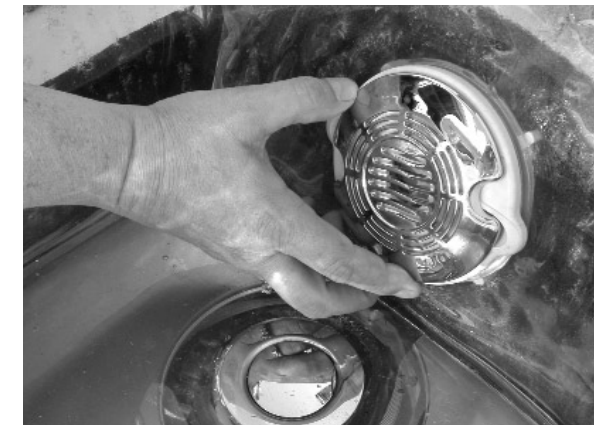
Replace screen by turning clockwise
